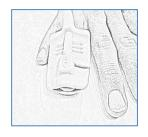
(!) Make sure your finger is inserted COMPLETELY! Your fingertip should touch the end of the sensor.
